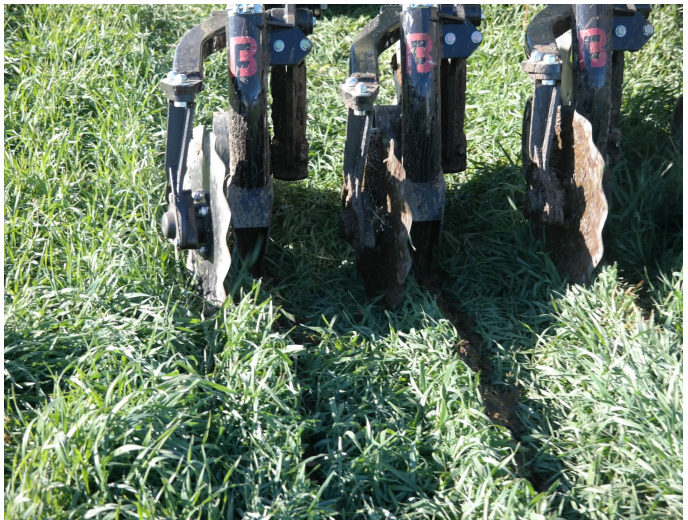
Rolling coulter manure injectors can fertilize established winter forage in the late fall, meeting all the nitrogen needs. Repeating the application after winter forage is harvested, can supply all the nitrogen for the following corn crop.
